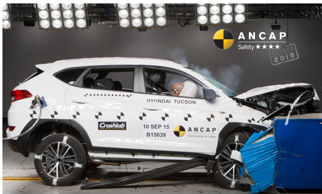
Frontal offset test at 64km/h
