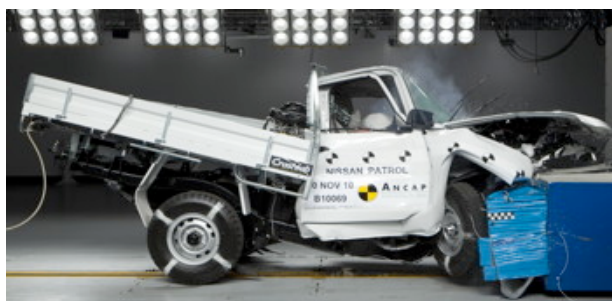
Offset crash test at 64km/h
