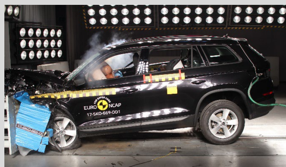
Frontal offset test at 64km/h
