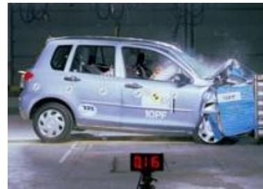
Offset crash test at 64km/hr
