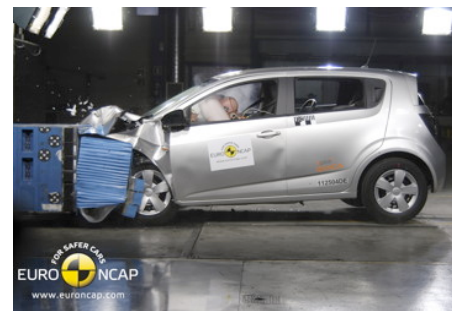
Frontal offset test at 64 km/h (Euro NCAP)
