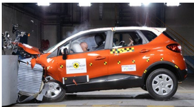
Frontal offset test at 64km/h (Euro NCAP)
