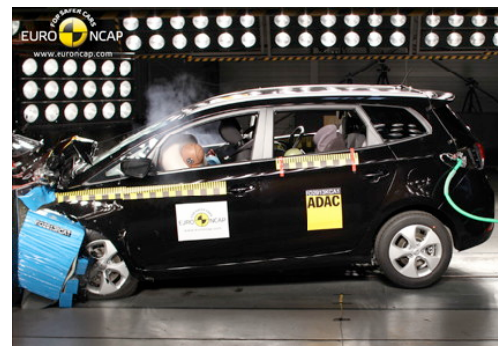
Frontal offset test at 64 km/h (Euro NCAP)
