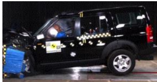
Offset crash test at 64km/hr
